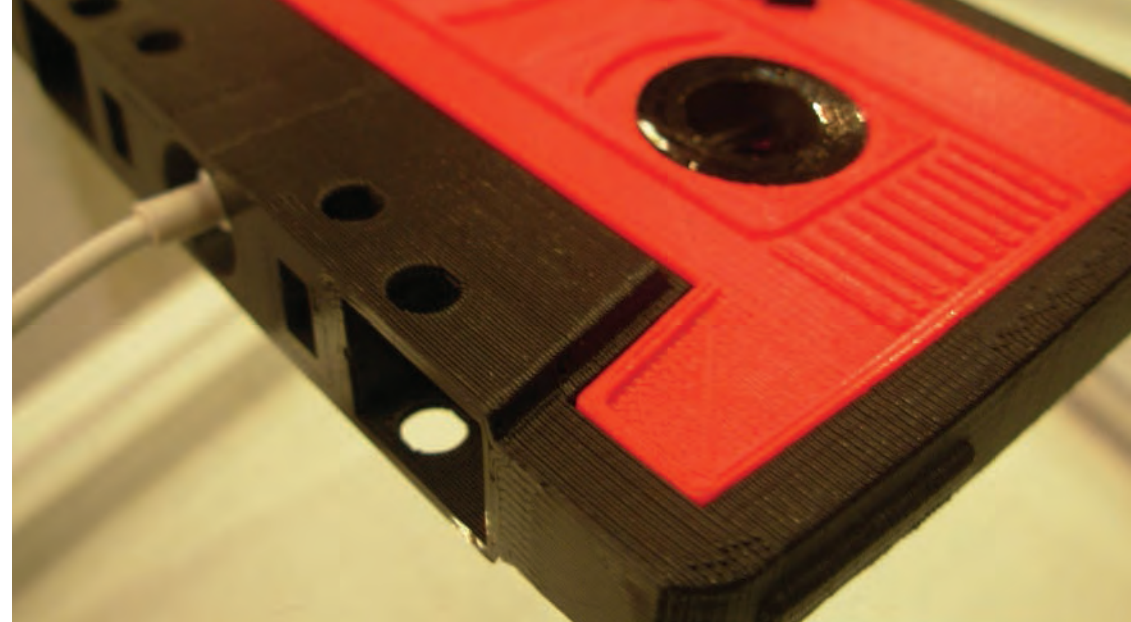
Photo: MakerBot mixtape printed using fused deposition modelling (FDM) © Econolyst
