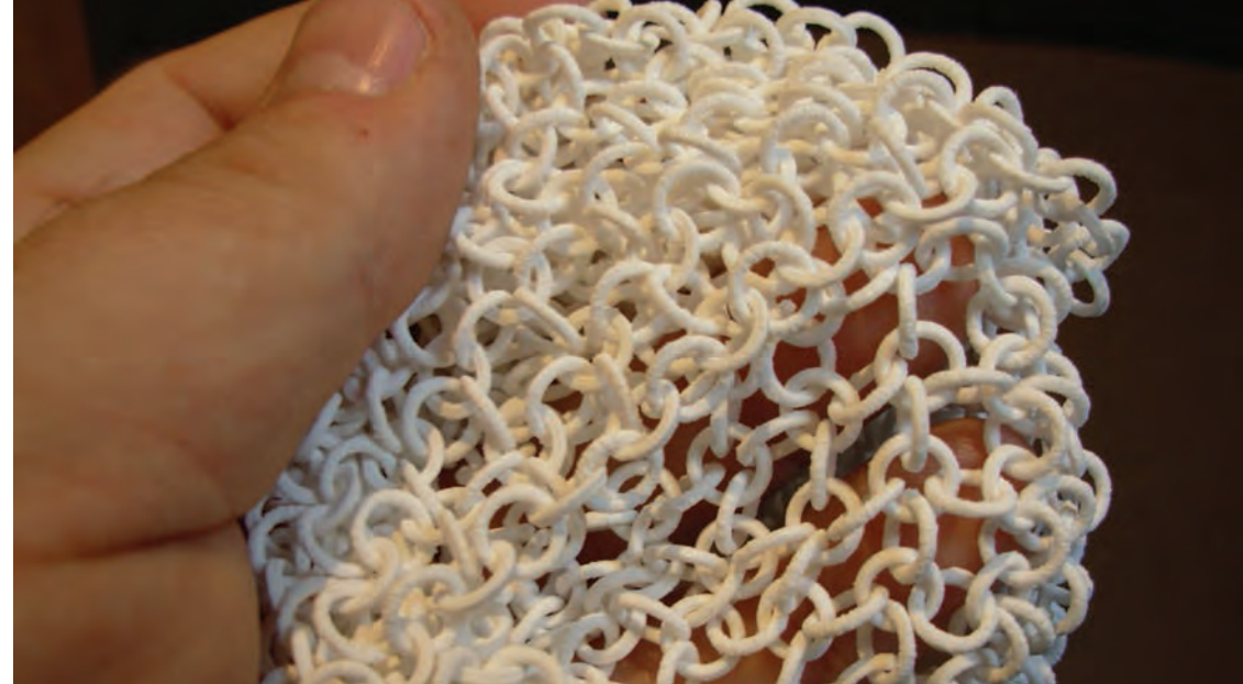
Photo: Selective laser sintered (SLS) chainlink © Econolyst
