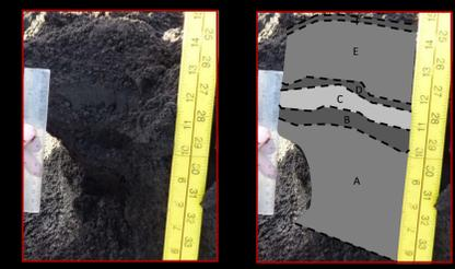
Figure 8: A cross section through the air-fall tephra on Sólheimajökull (Fig. 7) depicting the 6 layers sampled.
