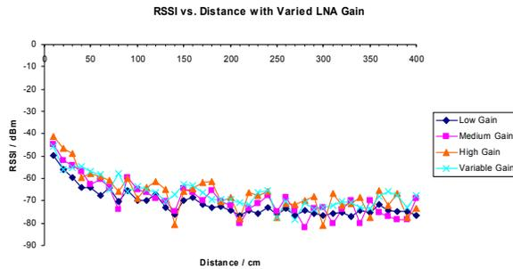
**Figure 8 – RSSI between two IEEE 802.15.4 nodes with 9dB attenuation on transmitter and varied LNA gain on receiver. Low std. dev.: mean 1.29dBm, max 2.72dBm, min 0.34dBm Med. std. dev.: mean 2.27dBm, max 4.54dBm, min 0.23dBm High std. dev.: mean 2.57dBm, max 6.65dBm, min 0.70dBm Var. std. dev.: mean 2.60dBm, max 5.51dBm, min 0.77dBm**
