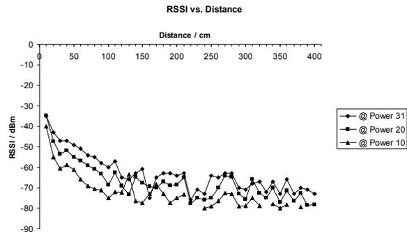
**Figure 7 – RSSI between two IEEE 802.15.4 nodes with 9db attenuation on transmitter and fixed LNA gain on receiver. Std. dev.: mean 4.52dBm, max 7.06dBm, min 2.20dBm**
