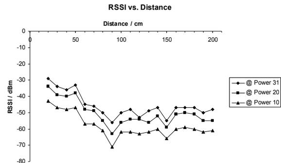
**Figure 3 – RSSI between two IEEE 802.15.4 nodes with factory default setting. Standard deviation: mean 10.32dBm, max 14.42dBm, min 6.61dBm**
