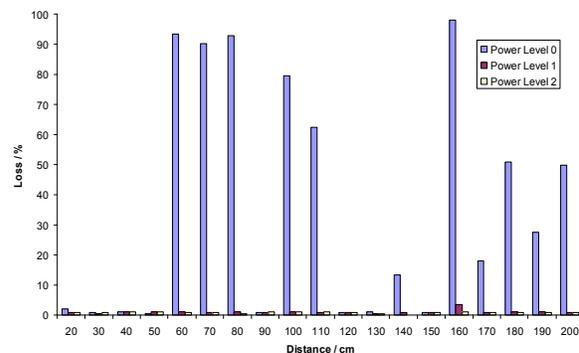
**Figure 4 – Packet loss observed between two IEEE 802.15.4 nodes with factory default setting.**
