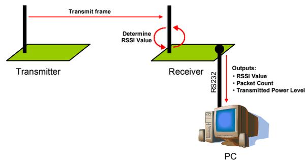
**Figure 2 - Experiment Configuration**
