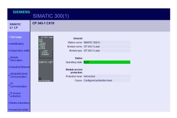
Figure 2: Siemens Simatic 300 Dashboard
