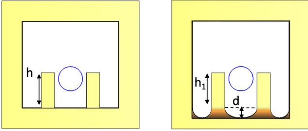
Fig. 2. Schematic of the original DCW (left) and modified (right) DCW including the cutting profile (the blue circle represents the electron beam).
