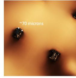
Fig. 4. Photo of the pillars realized by precision cutting.
