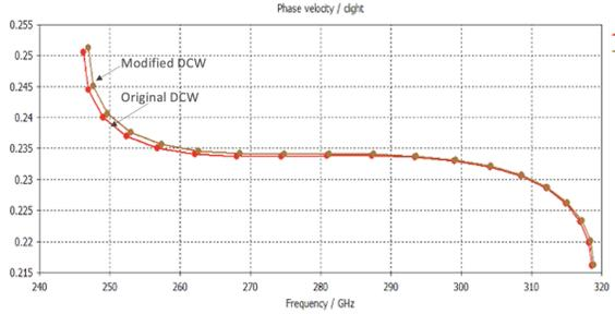
Fig. 3. Comparison of the dispersion curve of the DCW in Fig. 2.
