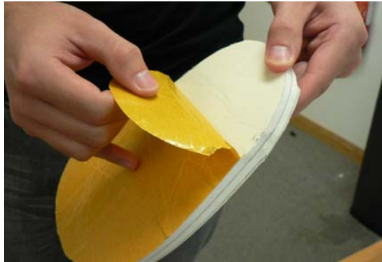
Figure 5.12: The adhesive backing can be used to stick areas of substrate to existing surfaces.
