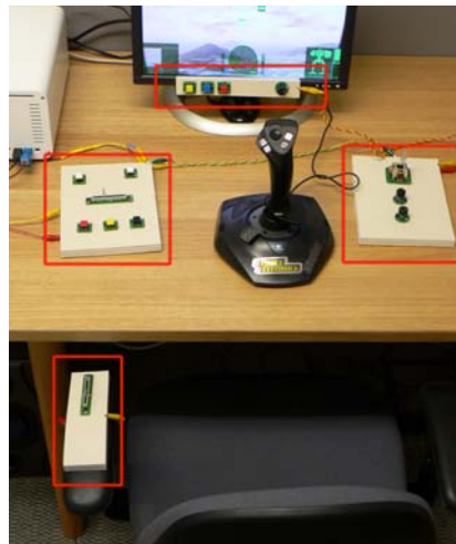
Figure 7.19: Cockpit design - notice how interface areas extend beyond the desktop to the monitor bezel and chair armrest.
