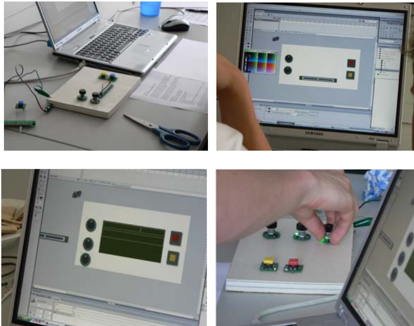
Figure 7.2: The participants initially moved from paper design and physical interface layout to work within Flash (top), and at later points introduced graphical elements first and then reflected and tested them on the physical stage (bottom).
