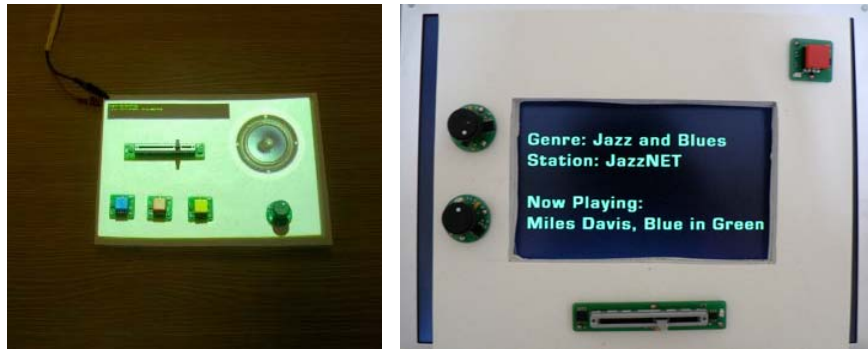
Figure 7.4: Integrating graphics by overhead projection (left) and a window cut-out (right).
