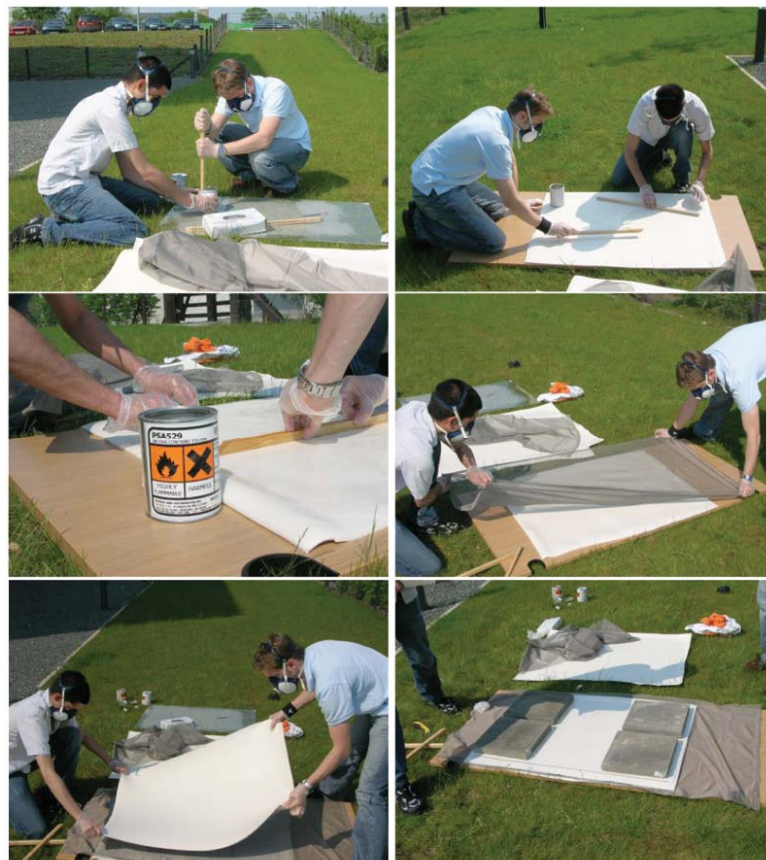
Figure 5.8: Substrate bonding process: layers of silicone foam rubber are alternated with layers of the conductive fabric, and bonded together using a silicone adhesive.
