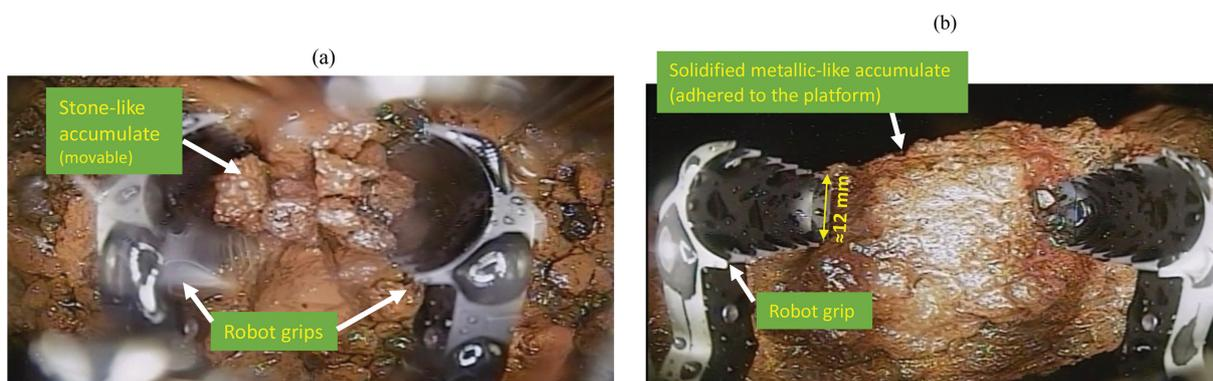
Figure 3. Investigation for the sediments (a) accumulated on the cable channel [17] and (b) adhered to the grating in the RPV pedestal [18].
