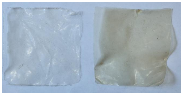
Figure 4 Image of pure tapioca starch film (left) and tapioca starch film with 5%(w/w%) olive stone powder (right).
