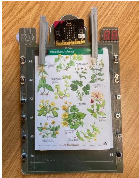
Figure 46 A prototype clipboard in cardboard with a 7 segment display and buttons
