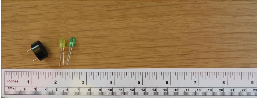
Figure 16 Common physical computing outputs: a buzzer and different coloured LEDs
