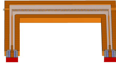
Fig. 9. Single-section ML-SWS with coaxial coupler at the input and output ports.
