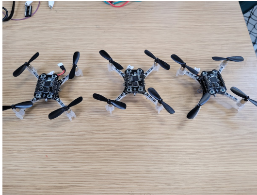
Figure 4.15: Three Crazyflie 2.1 nano quadrotors, equipped with Lighthouse Positioning Decks, used for real-world testing.
