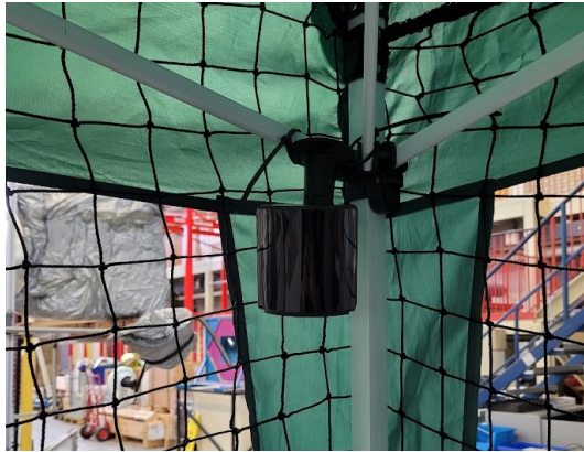
Figure 4.16: Photograph of the HTC Vive IR base station place in the test environment.
