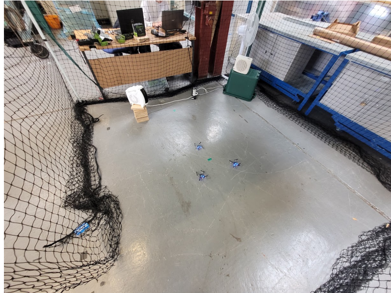
Figure 5.13: Test environment for data collection with two space heaters.
