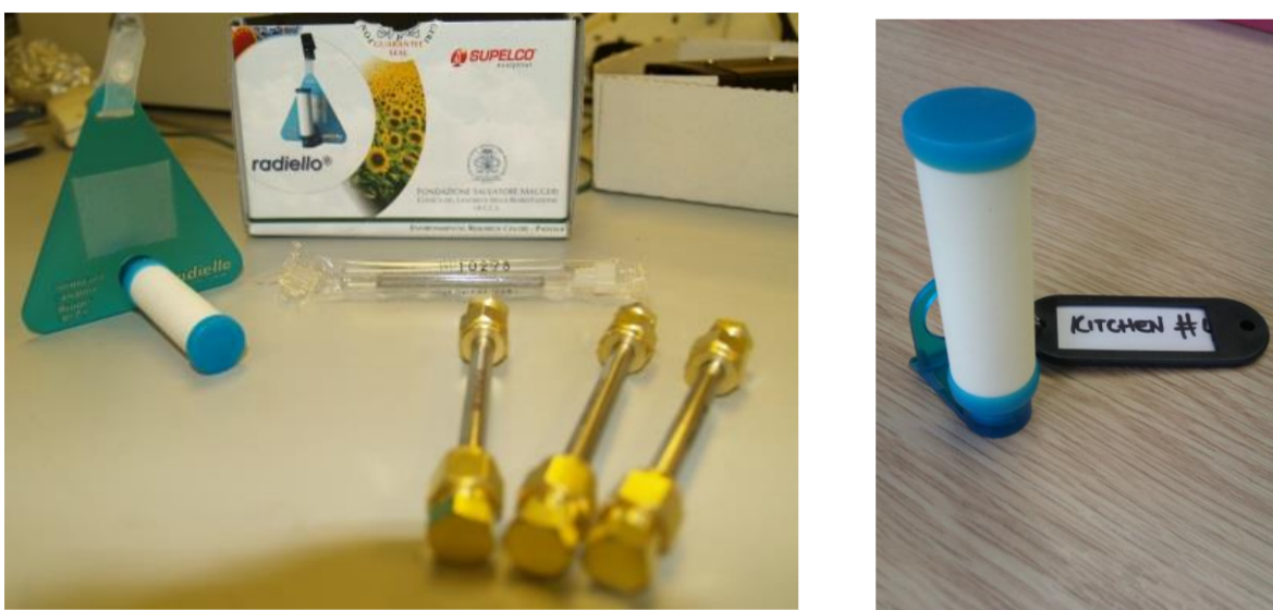
Figure 1: Radiello® passive sampling equipment. (a) cartridge, (b) mounted on vertical adapter for home sampling.
