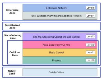
Fig. 1: The Purdue Reference Architecture for ICS [21]
