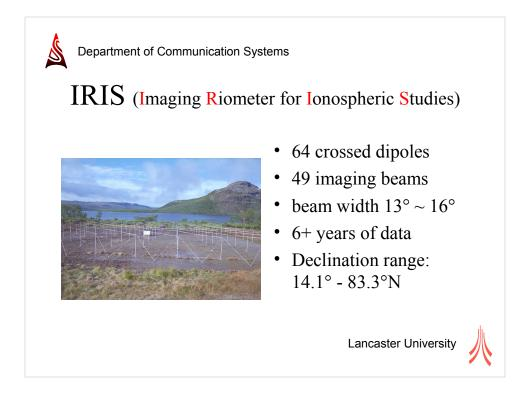
A riometer is designed to measure ionospheric absorption of radio waves by observing the deviation of received power from the expected level, or *quiet day curve*. By *quiet* I mean lack of particle precipitation, solar radio emissions and lightning.
