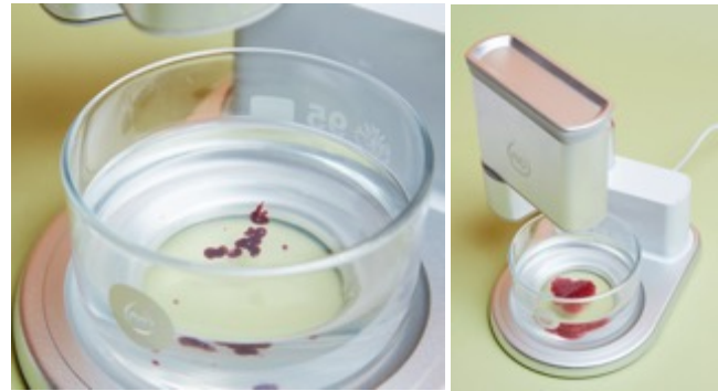
Figure 1. The nüfood printer during the printing phase (droplets of printed material can be seen in the bath on left)
