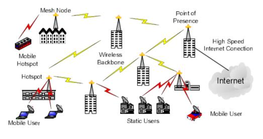
Figure 4 : WiMAX MESH Topology
