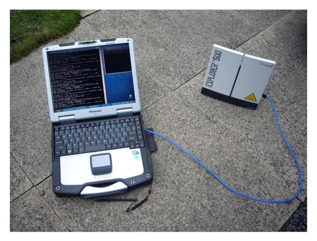
Figure 15 : Outdoor network tests of the Explorer 500 using a Panasonic Toughbook
