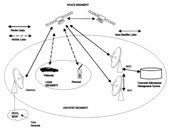
Figure 2 : Satellite Network Architecture [16]
